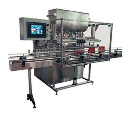
The REB IVS Series of automatic, in-line piston filling and depositing systems range from a single cylinder to a ten cylinders. Filling speeds range from 10 – 120 containers per minute.
