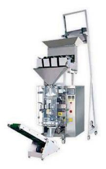
It's suitable for weighing slice, roll, or regular shape products such as sugar, salt, seed, rice, sesame, glutamate, milk powder, coffee powder, seasoning powder, etc.
