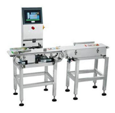
The weight checker is used to determine if a product meets the target weight, weigh materials, counts packs, and automatically rejects unqualified products. Users should choose the right weight checker according to the weighing range.
