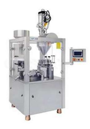
NJP-1200D automatic capsule filler processes the products for optimal productivity up to 1200 capsules per minutes, featuring low-maintenance operation, minimal downtime, and overall dependable production.
