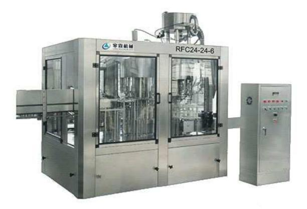
RFC - 3 IN 1 Series and RRFC - 4 IN 1 Monoblok Series machines are suitable for the production of Non Carbonated Beverages such as Drinking Water, Pure Water and Mineral water. The function of our machines would be Rinsing, Filling and Capping of bottles and our capacity range from 5000 bottles per hour to 20000 bottles per hour on standard 500 ml bottle size.
