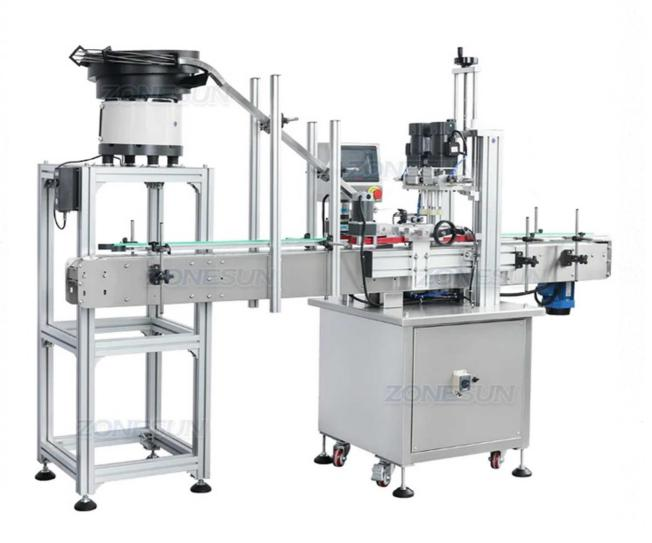
This automatic capping machine is good for various bottles like spray bottles, dropper bottles, trigger pump bottles. It is designed with bottle guiding structure, this is good for bottles that are easy to fall down during capping work, it can improve production quality. This machine is widely used in food, cosmetics, daily chemical industries.
