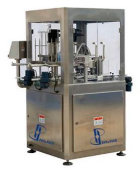
A can seamer machine is used to hermetically seal a lid to a can body during the packaging process using a double, or sometimes triple, seam. The lid is usually made from tin-plated steel. Meanwhile, the can's body can be made of paper (like whiskey cans), tin, aluminum, PET, plastic, or glass. The formed seam is usually leak-proof. However, this still depends on the type of products being packaged.
