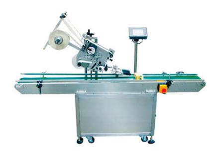
This machine is designed for labeling on flat surface
