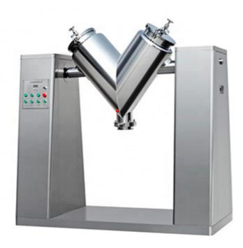
This machine is widely used for mixing powder and granular materials in pharmaceutical, chemical, feed, metallurgy and other industries.
