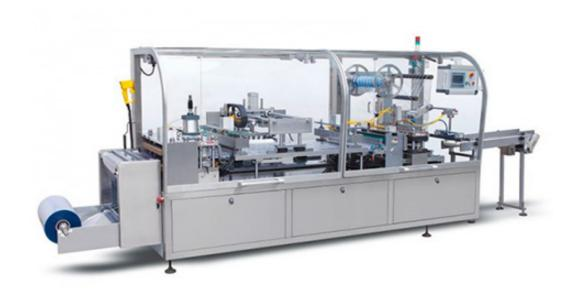
The machine suitable for syringe, ampoule, vials and bottle, medical appliances, battery and other special shape products Alu-PVC packing.
