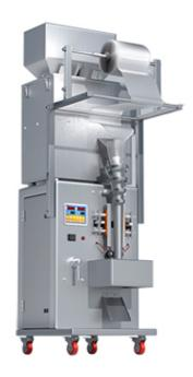
The 2-head 100g electric small packaging machine produced by Jieding is suitable for quantitative, weighing, filling, and sealing of particles, powders, and materials such as rice, millet, grains, vegetable seeds, cat food, dog food, fertilizer feed, nut seeds, corn seeds, coffee beans, coffee powder, flour, pepper powder, seasoning powder, etc.
