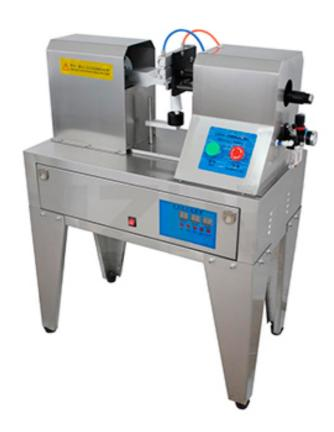
Ultrasonic plastic tube sealing machine is suitable for toothpaste, cosmetics, medicines, food tube sealing.
