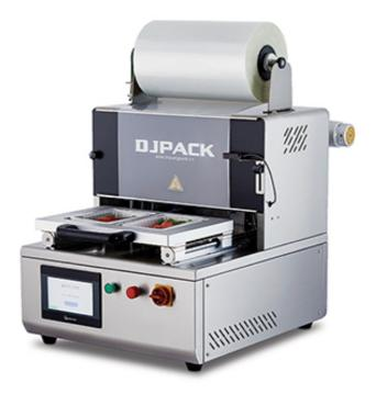
The DJT-400G Tabletop MAP Tray Sealer allows trays to be packaged in a very limited space and can thus be used in a versatile manner. It's an economical solution for the packaging of small batches. The DJT-400G is operated slowly by electricity, it can be individually equipped. It's widely applicable for the package of raw and cooked meat, seafood, dairy product, fruit and vegetable, rice and food.
