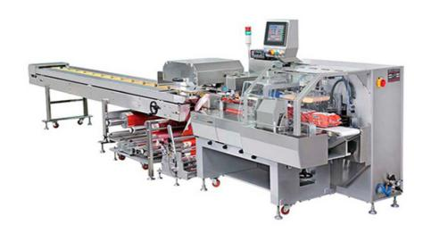
The frozen food packaging machine belongs to the down film type packaging machine, which is designed for the high product, secondary package, group package, or family package. The multipack biscuit packaging machine controlled by 5 servo motors can pack multi-bags.
