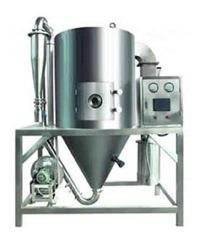
Centrifugal spray dryer is suitable for drying emulsion suspending liquid, liquor and so on. Particularly it has unique advantage for drying polymers and resins; dyestuff and pigment; ceramics, glass; derust agent; pesticide; carbohydrate, dairy products; detergent and surfactant; fertilizer, organic compound, inorganic compound and so on.
