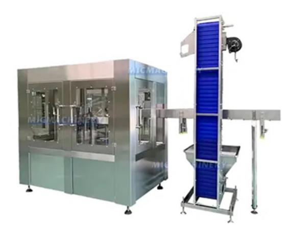
MIC12-12-5 juice Bottle filling line is a kind of professional filling machine for mango juice, litchi juice, orange juice, apple juice and other Fruit and vegetable juice reduction. It is made of high quality SUS304 stainless steel. Main components are processed precisely by CNC machine tool. The machine adopts advanced photo electricity to detect running status. No bottle no filling. It realize man-machine conversation because of applying touch screen for operation
