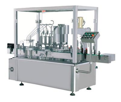
Automatic Filling and Capping monobloc is customized for bottle liquid filling and plastic screw cap capping (alternative alum. seaming). The machine is composed by a wide in-feed conveyor, SS316L volumetric piston pump with servo system, track top-bottom filling nozzles, liquid buffer tank, bottle index wheel sets, rotary turret, capping assembly etc.
