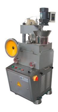
This machine is used to press the granular raw material into the round tablets or various geometric shaped tablets, it is especially caters for small scale production. When pressing the tablets, the rotary disc speed and filling depth of material can be adjustable.
