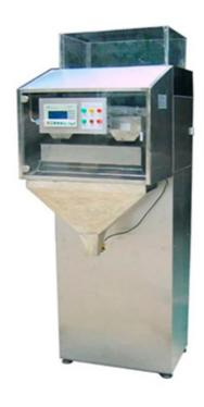
Automatic electronic weighing filling machine adopts electronic balance weighing, Microcomputer control and twin vibrator filling, and it with stainless steel structure, manual bag feeding and automatic weighting, It is used to weigh objects in grain or powder shape with good fluidity.
