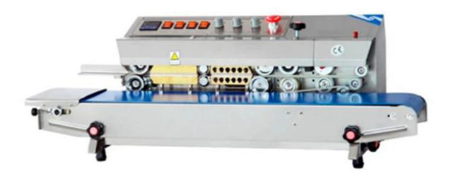
FRM-810I feeds from left to right and equipped with a hot ink coding imprinter to print a date, expiration date, or lot code.
