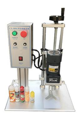
Manual press is set on the plug, cap by hand, out of the bottle in an ideal semi automatic machinery,
