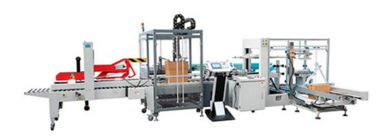
The machine is suitable for paper carton erecting automatically. It has function of cover-folding, sealing bottom with tape. It is economical and it is with high high-efficiency. It is ideal automatic carton forming and bottom sealing equipment.
