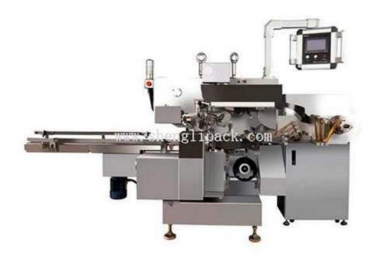
SL-SBJP260 series packing machine is designed for bottle shape solid chocolate and liqueur chocolate. The packaging adopts aluminum foil single-layer packaging and the unique design and process ensure consistent packaging performance and perfect fit.
