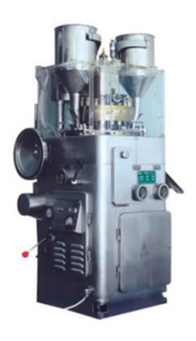
Double layer tablet press is a kind of automatically revolving and continuous tablet press machine. It is the essential equipment to press granular materials into tablets in pharmaceutical, chemical, food and other industrial sectors. ZPW21B is an improved version of ZPW21A. These double layer tablet presses can press not only round tablets but also tablets in different geometrical shapes. The tablets may have letters on both sides.
