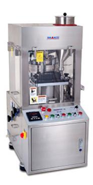
Lab Press LP- II is a High Tech Rotary Tablet Press in table-top design for R & D and small batch production. This Single sided R & D Tablet Press fully conforms to GMP and the safety requirements. All Electrical settings can be performed by Front panel with indicators at the front of the machine. The machine is equipped with pre pressing and main pressing systems. The compression force can be adjusted up to 6 tons.
