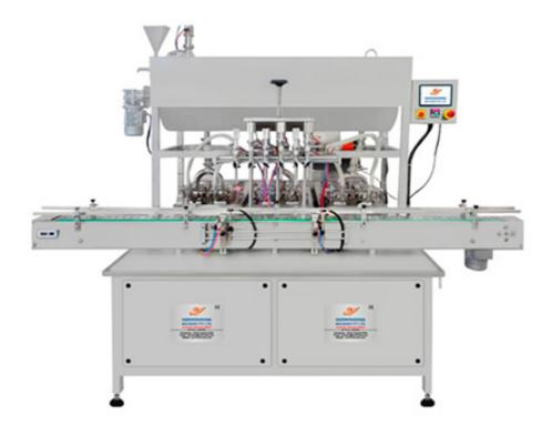
The Automatic Piston Filling Machine consists of a main structure, product transmission belt with an adjustable guide, jacketed storage tank for filling material, safety polycarbonate enclosure with SS pipe frame (OPTIONAL), pneumatic bottle stopping facility, pneumatic operated filling nozzle, electrical panel, motor, sensor, PLC & HMI, AC drive & mains ON/OFF.
