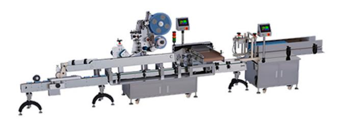
This series of products integrates the whole line of labeling, palletizing, and linkage control. It is suitable for high-speed automatic labeling and feeding of various oral liquid bottles, ampoules, vials, etc.
