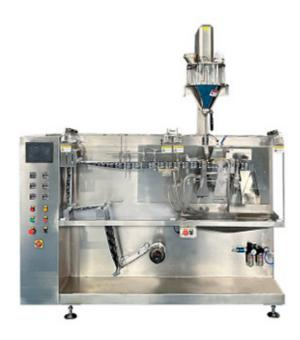
HC-110 horizontal packaging machine is an ideal bag packaging equipment that meets the requirements of high-quality packaging and smaller bags. The packaging speed is fast, and it can realize three-side sealing and four-side sealing bags; Packaging needs for various materials such as body and solid objects; roll film forming is used to reduce packaging costs.
