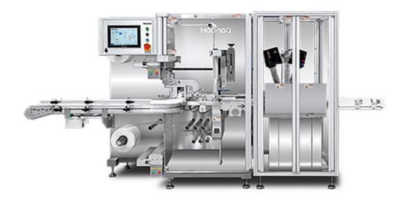
HB 40B is a specialized shrink-wrapping machine for bundle packaging which meets GMP compliant design through servo motor driven system. Instead of applying heat-shrinkage tunnel, products are gently wrapped through hot-wind system. This high level of technology offers remarkable performance and reliability as end-of-line packaging.
