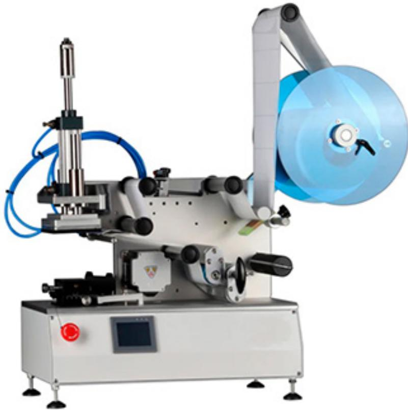
This semi-automatic flat surface labeling machine is designed for accurately applying labels on flat or slightly curved surfaces, making it suitable for a wide range of products such as boxes, bags, lids, containers, and more. It's commonly used in industries like cosmetics, food, pharmaceuticals, and electronics, where precise label placement is critical for product appearance and compliance.
