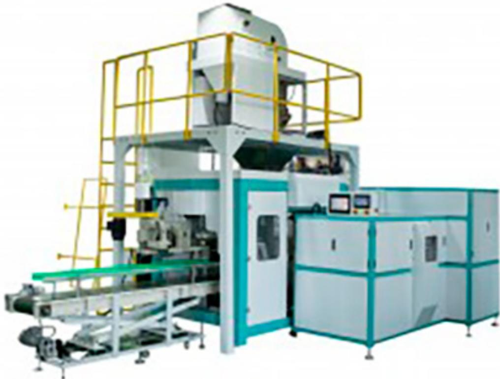
Fully automatic packaging machine, after the equipment is manually placed in the bag roll, it can realize automatic bag making, automatic bag supply, automatic bag loading, automatic bag opening, automatic detection, automatic weighing, automatic filling, automatic packaging, automatic label delivery, high degree of automation.
