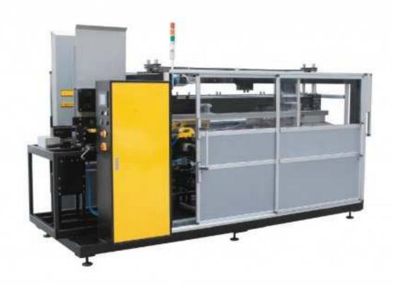
Case equipment is used to erect, pack, seal, or unpack cases of products. In most instances, case equipment is used to form cardboard boxes; however, corrugated materials and plastics formers are also available. Types of case equipment include case erectors, case cartoners, carton packers, carton sealers, and unpackers.
