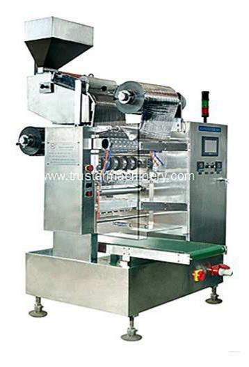
This machine suitable for the medicine and food industrial .It can pack tablet in the normal or special shapes, also capsule and the solid state product. It is small occupation, running stably, high capacity etc.
