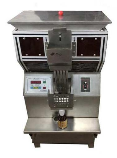
It is a professional hard capsule counting machine, which also equipped automatic counting machine. It has features of operation and the counting speed can be adjusted by manual loading the bottle speed. The bottle will stop counting when the one bottle is full and it can start counting when empty bottle is loaded.
