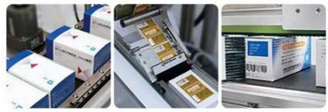
A741 is a flexible system that can label on the top or the side surface of the packaging. Various functional components such as separation wheel, hold-down belt, inspection and rejection mechanism etc. can be flexibly integrated into the system to meet different application requirements. Optional thermal transfer print engine to print and apply variable data and barcodes on line, which is an excellent companion for the PIATS applications.
