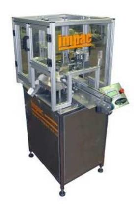
The Cyclone series was designed to give a solution for filling glass ampoules with liquids and sealing them by fusion using profane gas burner.
