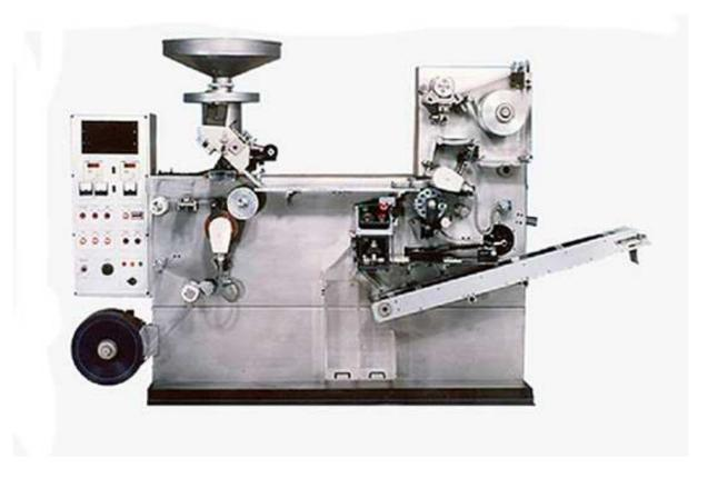
The PEW-RP-240 is an automatic Blister Packaging machine utilized for packaging of the tablets, capsules in a blister pack.
