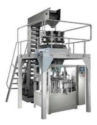
Model AP-600P-Up to 5 TracksB can operate at a maximum speed of 60 SPM and is efficient in packaging up to 200 grams of free flow powder and granules. Depending on the width of sachet or pouch, these machines are provided with maximum 5 tracks. To ensure safe packaging, this model is offered with 4 side sealing. These machines are constructed using superior quality of stainless steel with powder and SS coatings.
