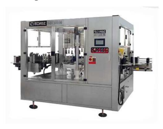
This machine is fully automatic rotary servo positioning self-adhesive labeling machine. Used for different industries for beer, white spirit, seasoning, soft drink, mineral water, cosmetics, cans and others. It has the advantages of humanized design, flexible and convenient adjustment, easy to operate, low speed and large torque, clean labeling environment, high stability. It's the necessary labeling machine for the company to upgrade their product and quality.
