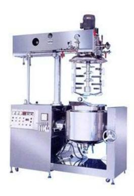
This machine is composed of one blade mixer for high viscosity and one micro homogeneous high speed mixer with high strength-cut-off.
