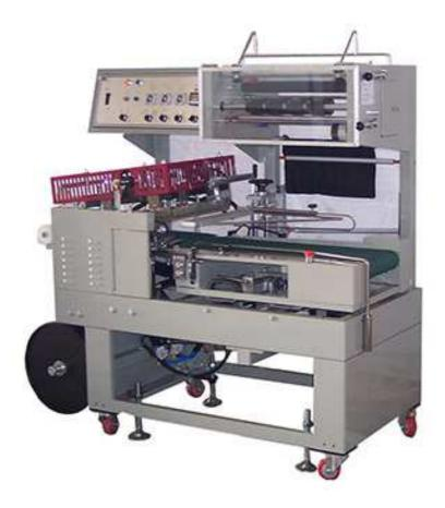
TAYI YEH TY-700-80S Auto L-Sealer offers best effective and economical output. Equipped with closing conveyor, TY-700-80S is ideal for compact or multi-shape packages. High speed continuous production process capacity of up to 25 PPM
