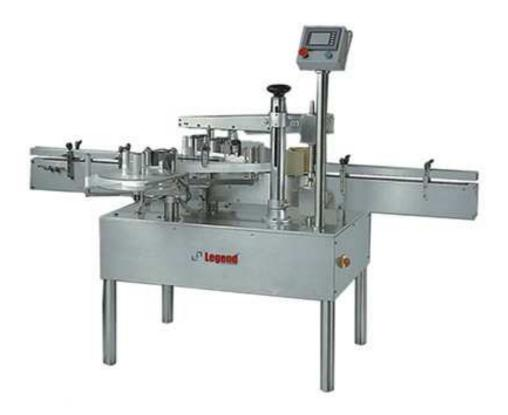
A versatile, elegantly designed linear labelling machine Suitable for applying Front, Back or Side Labels on Flat/Oval/Square shape containers with output ranging from 50-120 Labels per minute depending on products Shape/Size and label size.
