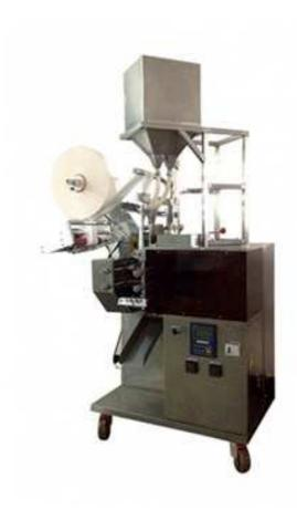
It is suitable for packing products with granule or powder shape.
