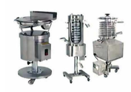
We have been supplying a qualitative range of De-Dusting & De-Burring Unit for our clients. It is precisely designed as per GMP guidelines at our unit making use of high grade stainless steel. This makes all parts of our De-Dusting & De-Burring Unit easy to wash and clean. Our offered unit is suitable for all types of tablet press machine. We have gained huge appreciation for its noiseless operations, low maintenance, effectiveness and a long operational life as tested by our experts.
