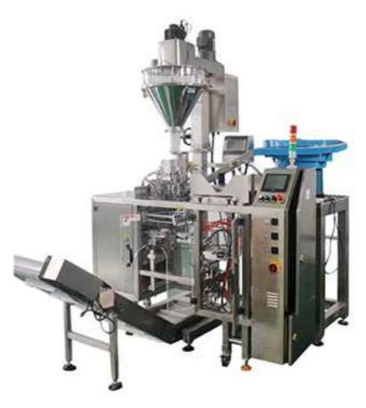
This machine completes the whole packing procedure of measuring, loading materials, bagging, date printing, charging (exhausting) and products transporting automatically as well as counting can be used in powder and granular material: like milk powder, Albumen powder, solid drink, white sugar, dextrose, coffee powder, and so on.
