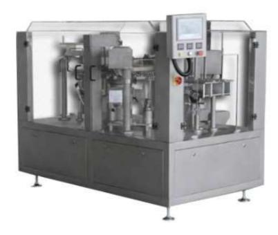
Automatic rotary packing machine SR300 is designed for pre-made bags with many expected bag styles. From manually place stacks of pre-made bags on the bag feeder, it will automatically open the empty bags, fill, seal, print then convey out.
