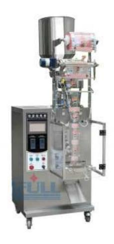
SF-220G Small Granule Packaging Machine is suitable for pharmacy food, household chemicals, plastic products and other special industry and other loose type and in viscid granule material Such as seeds, Chinese Drugs, feeding stuff, medicinal, granules, puller, monosodium glutamate, salt, sugar, soup blend, oat, tea, active carbon, washing powder, dryer, etc.
