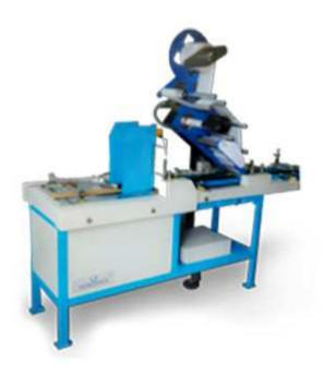
Worldpack Pouch Labelling Machine made of 304 stainless steel is extremely durable, versatile and compact. It allows single side and dual side labelling for pouches of various sizes. Depending on output requirement the machine can print 40 to 60 pouches per minute. It has a maximum label roll diameter of 300mm and max length of 150mm. It is also equipped with a 3m long conveyor.
