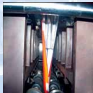
Die-based Sealing that integrates both Horizontal & Vertical Sealing.
