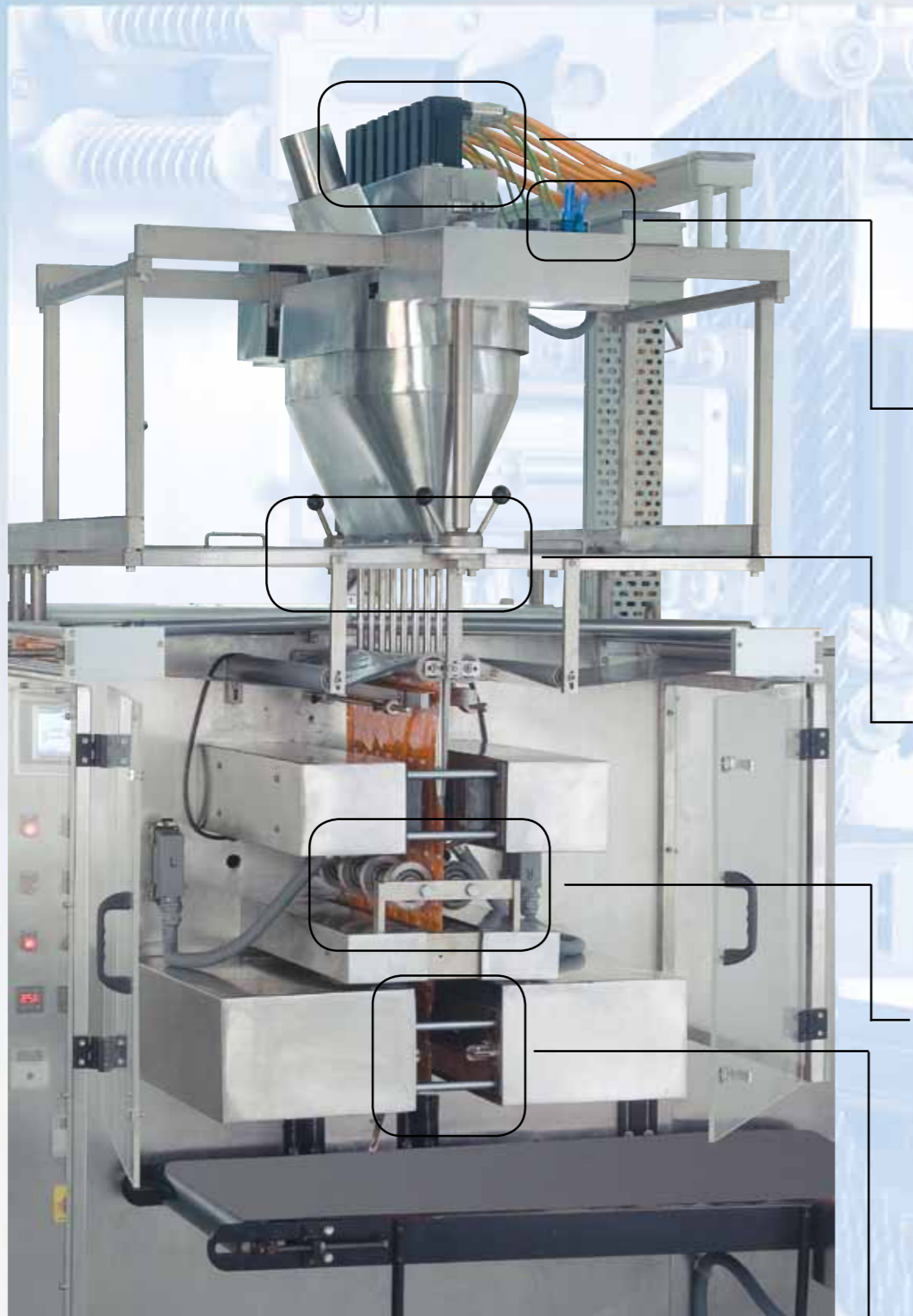
Independent Servo motor driven Auger Screw for each lane.
