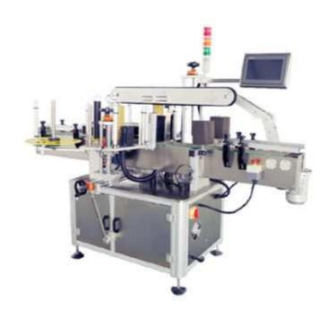
A labeling machine or label applicator, is a machine that put the label on the product and wipe on to assure adhesion. The labeling machine is popular in these area, such as bulk mailing, manufacturing, packaging, food and beverage, fast food, photo labs, and more.
